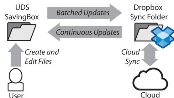
Fig. 2: High-level design of the UDS middleware
