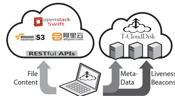
Fig. 3: T-CloudDisk system architecture
