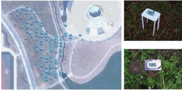
Fig. 13. The deployment and enclosure of motes.
