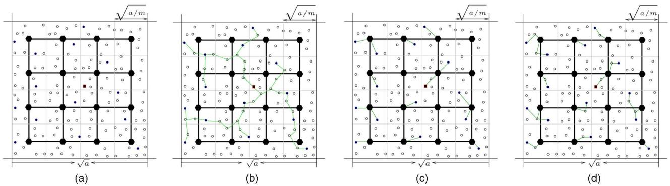
Fig. 1. Illustrations of three types of multicast routing schemes. The small hexagons represent the base stations that are assumed to be connected via the high-bandwidth wired links. The cases that  $a = n$  and  $a = 1$  correspond to the *hybrid extended network* and *hybrid dense network*, respectively. (a) Original network. (b) Ordinary ad hoc strategy. (c) BS-based strategy. (d) Hybrid routing strategy.
