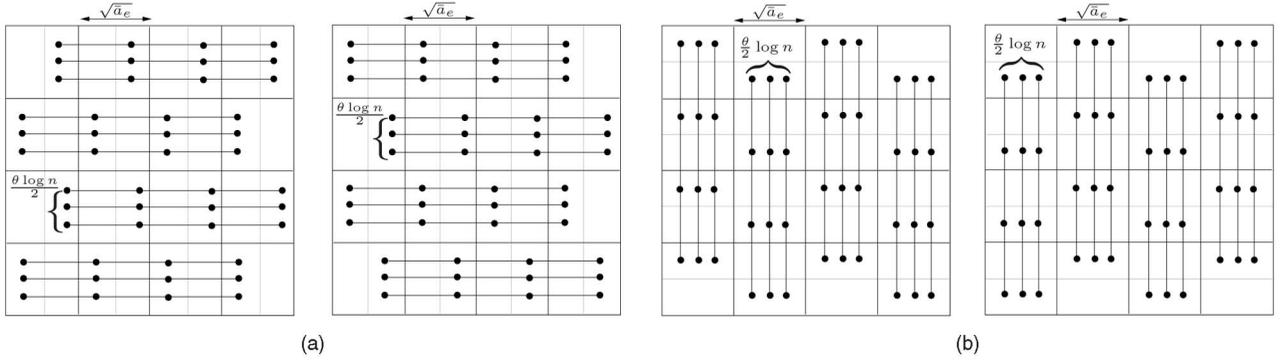
Fig. 2. Construction of connectivity paths. There are at least  $\theta \log n$  connectivity paths, represented by the chains, in each column or row. (a) Horizontal parallel connectivity paths. (b) Vertical parallel connectivity paths.
